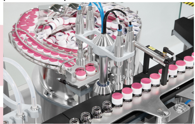
Figure 5: A typical vial fill line
